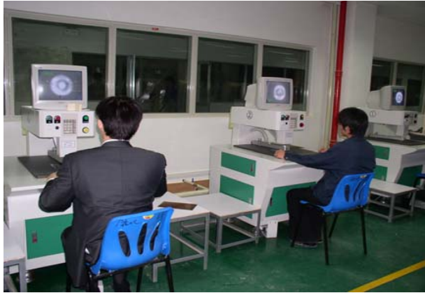
Punching Guild-holes Drilling ( leaser positioning)
