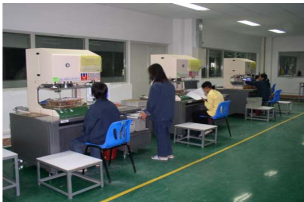
Electrical test O/S
